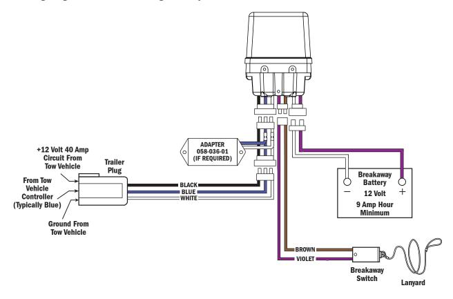
Figure 3: Wiring Diagram for BrakeRite SD Actuators:
